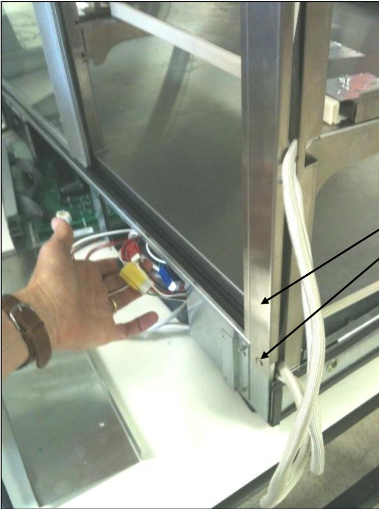
Removing this screw will allow this trim to move for easier cable access.
