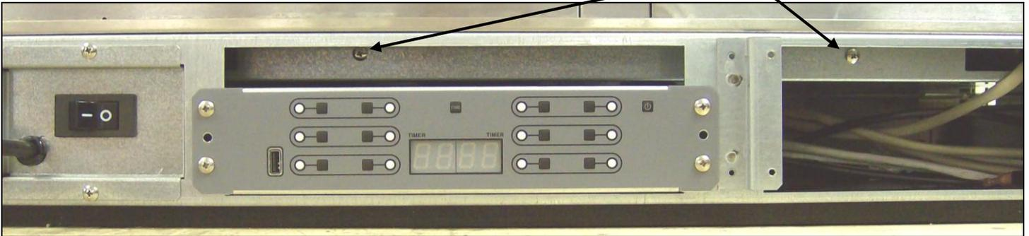
**Step 11:** Open the front of the HFD and remove these three screws.
